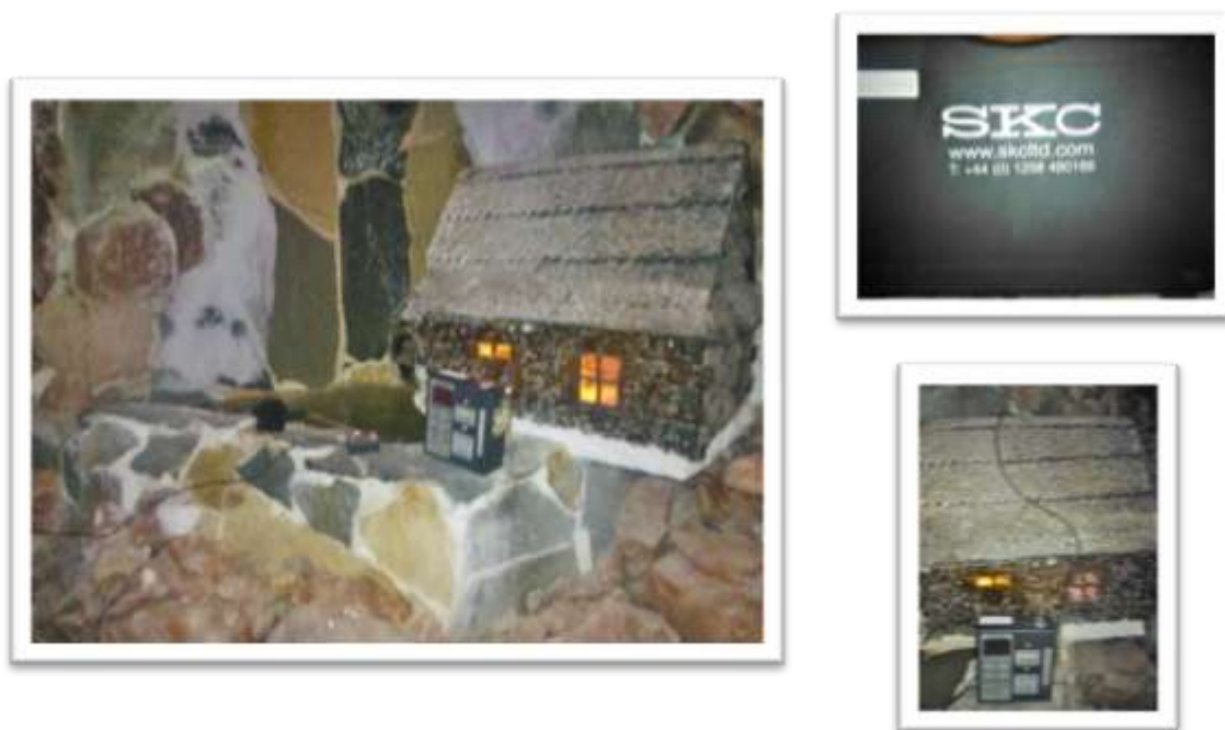
Photo 3. The sampling set up inside the Crystalotherapy Salt Cave salt (pump on the cascade).
