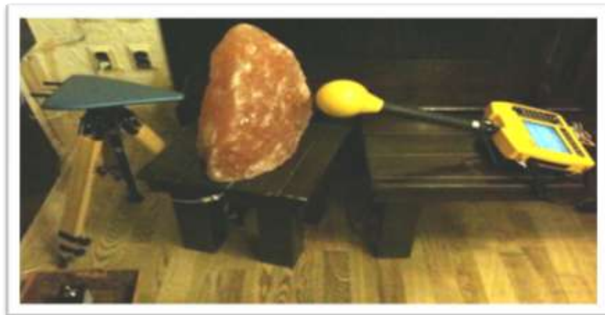
Photo 5. Spectrum analyzer with tixial probe (receiver) to the right and transmitter (RefRad 3000 reference source with directional antenna) to the left of the salt rock.
